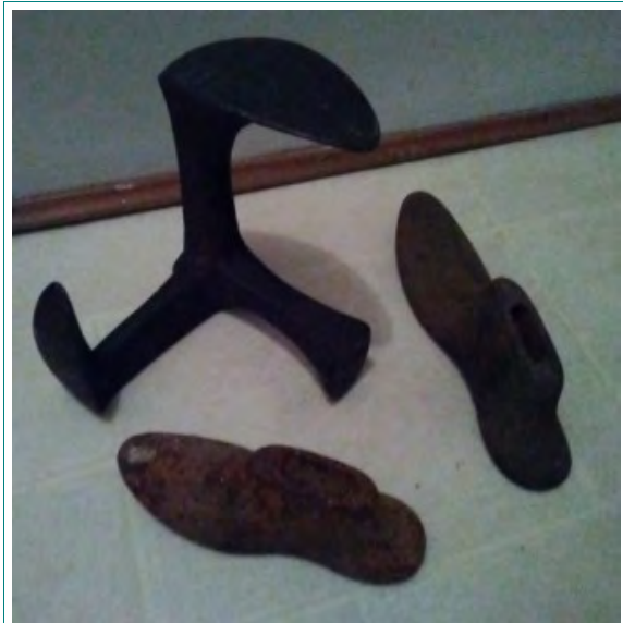
This pair of "lasts" were used to make shoes. The tall lasts were used for shoe repair
